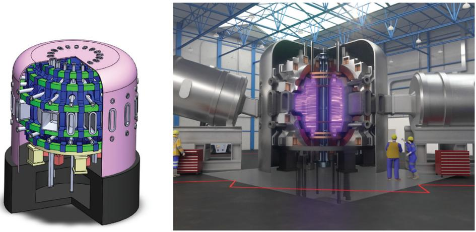
Fig. 5. Three-dimensional computer-aided design renderings of the baseline EXCITE design point showing all major subsystems, including superconducting CS and TF coils, copper divertor and vertical stability coils, double-walled vacuum vessel, cryostat, gravity supports, and auxiliary infrastructure. While the neutral beam H&CD is not explicitly considered in this study, this design does allow for the possibility of multiple beam lines.
